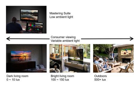
While mastering suites maintain low light (top), the ambient light levels in consumer viewing vary tremendously (bottom).
