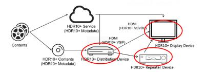
HDR10+ certification covers "distribution" devices like set top boxes and Blu-ray Disc players and "repeater" devices like AV receivers as well as "displays."
