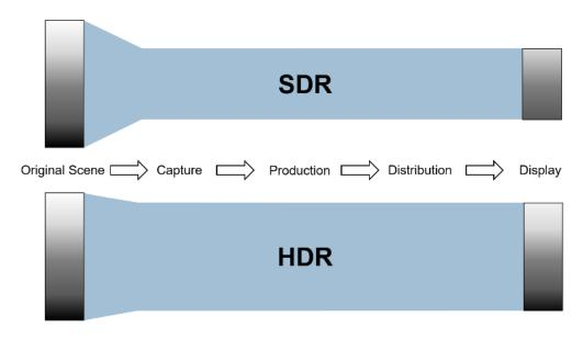
SDR (top) doesn't come close to the full range of brightness we can perceive in the original scene. HDR (bottom) does.
