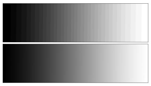
At the top, the distracting stripes of tone constitute "banding." At the bottom, superior grayscale enables a smooth transition from dark to light.
