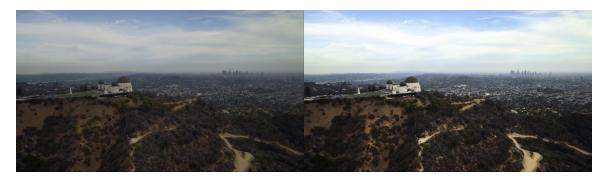
On the left, tone mapping with static metadata. On the right, HDR10+guided tone mapping with dynamic metadata.
