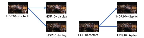
At left, HDR10+ displays realize the full benefit of HDR10+ content, which also works seamlessly on HDR10 displays. At right, HDR10+ displays support HDR10 content as well.
