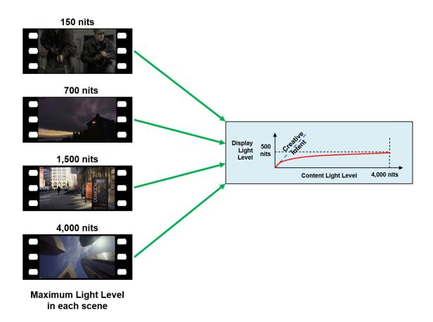
Maximum light levels vary from scene to scene. For example, highlights in the skyscraper scene at the bottom extend to 4,000 nits. Static metadata generates a single tone mapping curve based on the maximum light level in the entire program.
