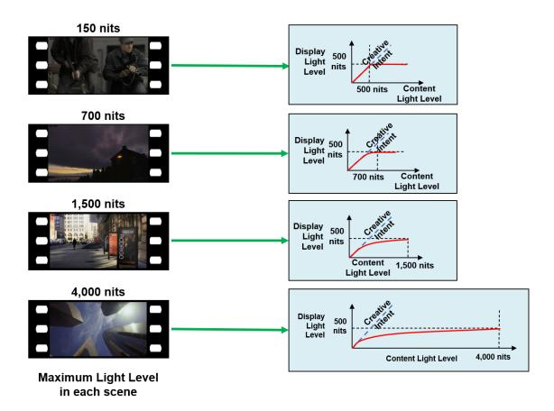
In contrast, dynamic metadata indicates the maximum light level for each scene, enabling the display to optimize the tone mapping curve on a scene-by-scene basis. You get a closer match to the creative intent line in low-light scenes, delivering much more detail in the shadows.
